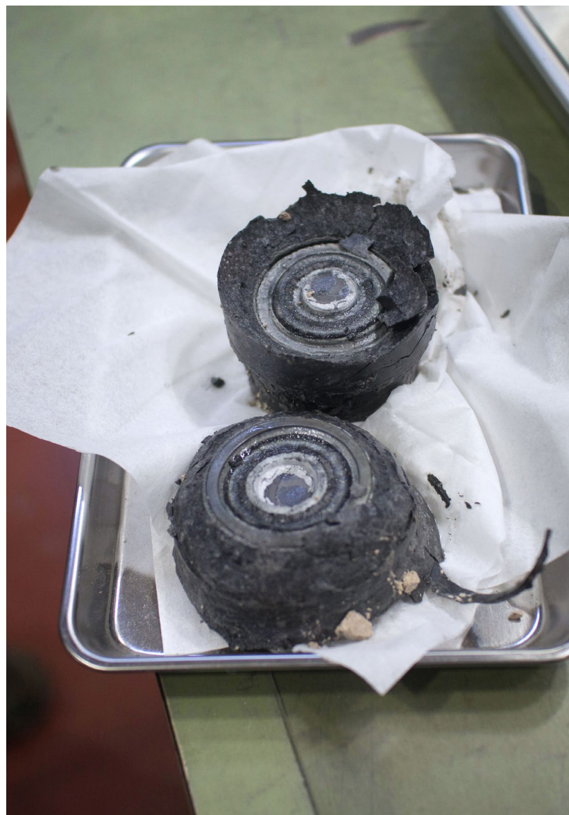
The synthesized hBN crystals, together with uncrystallized boron nitride powder, are contained in a molybdenum capsule.
